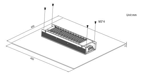
2. For heat dissipation, at least 5cm installation distance around the PSU should be kept, shown as below:
