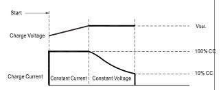
O Apply to Lead-acid batteries
